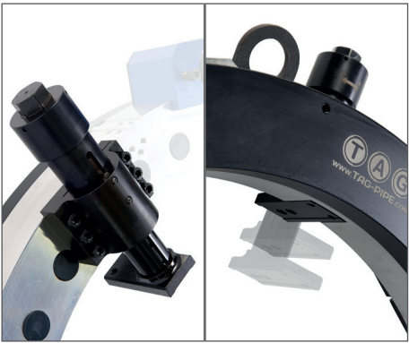
Individual movable telescopic locking system externally mounted to keep aluminium ring solid for extra strength, increased clamping foot size 55 x 115 mm for fast accurate setup.
