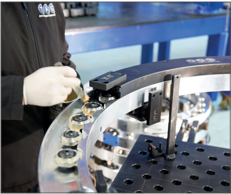
TAG advanced cam roller bearing system enables fine adjustment of bearings for optimal performance and maintenance delivering smooth precise rotation.
