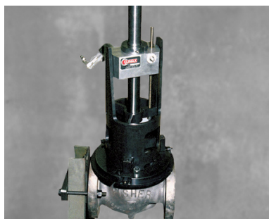
VM8000 Globe and Control Valve Repair
