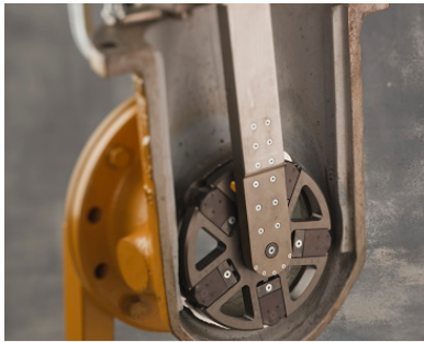
VM1000 Gate Valve Repair
